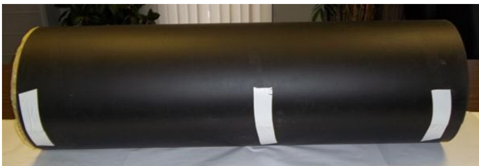
Figure 4 – Mass loaded vinyl secured lightly with tape.
